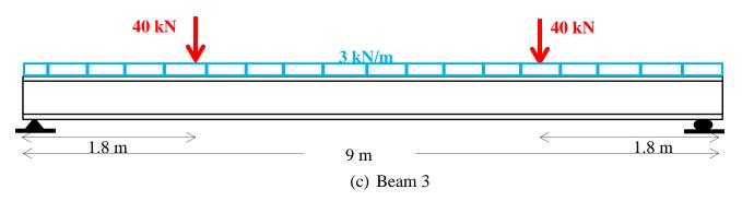
Fig. 6. Loading on beams used in case study
