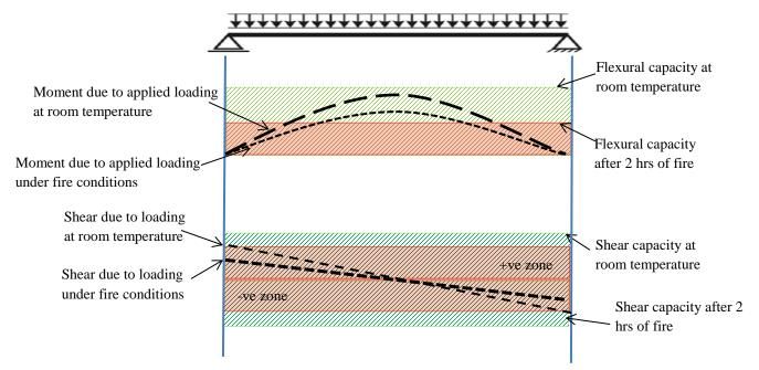
(a) Beam with uniformly distributed loading at ambient and fire conditions
