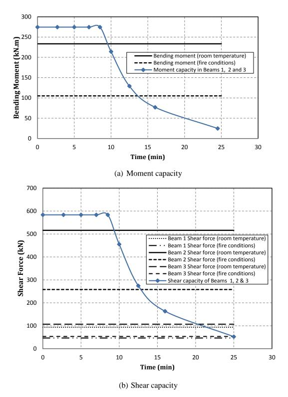
Fig. 8. Degradation of bending moment and shear capacity with fire exposure time
