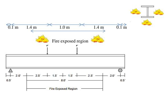
Fig. 3. Tested beam used in validating the developed finite element model
