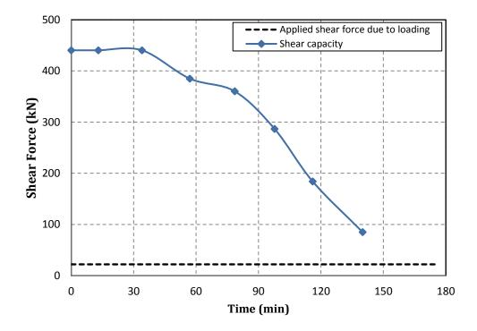
(b) Shear capacity Fig. 5. Degradation of moment and shear capacity in the tested beam [10]
