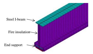
Fig. 13. Detailed view of fire insulated steel "Beam 6"
